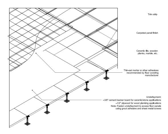
Routinely the need arises, in certain areas of the building, to place a speciality floor finish such as marble, granite,ceramic,wooden planking, etc. on top of an access floor system. Generally these areas (lobbies, bathrooms, cafeterias, wet areas, etc.) do not require complete access or any access to the floor system. When this need arises, consider the following detail.
